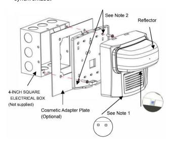
Note 1: To remove the cover, depress the snap at the bottom of the product with a key (or flat tip screwdriver) while fulling the cover up with the other hand.
