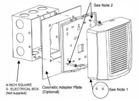
Note 2: The product attaches directly to a standard 4-inch square electrical box (not supplied) flush mounted or surface mounted. Attach the product to the back cover using two screws (supplied) mounted.
